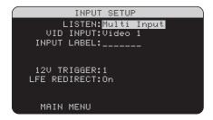
When the MULTI INPUT source is selected on the INPUT SETUP menu, the available options change to reflect the fact that these inputs are direct analog inputs and bypass the RSX-1067's digital processing. The INPUT, CINEMA EQ, and DEFAULT MODE options are not available since these are all digitally implemented features.
